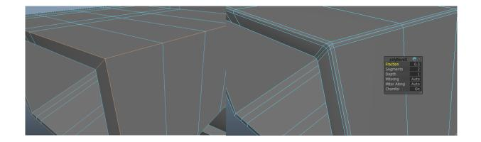
The correct way to go about having bevels with equal fractions in relative space is to do them all at once. This time, I've selected both sets of edge loops and slapped a bevel on them, using the same values as always. The bevels work great now, and the end product is what I was looking for!
