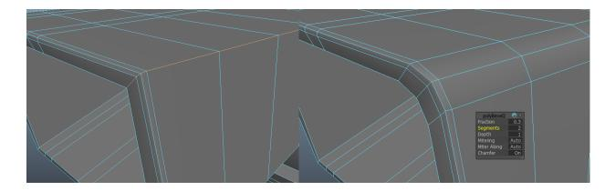
However, if we do the same exact thing to the intersecting edge loop, using the same 0.3 and 2 values, we get a monstrosity that's far too thick. This is the bevel tool freaking out because both bevels were done at separate times.
