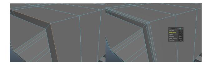
In this example, one edge loop is selected and beveled. The values for this bevel are 0.3 (fraction) and 2 (segments). The resulting bevel is looking fine!
