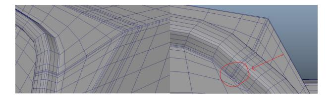
Here we see one of the unintended consequences of sticking edge loops in a high-poly model without being careful. The supporting edge loop is necessary for the upper corner of the model to remain rigid, but it loops over to this corner and creates a weird piece of geometry.
