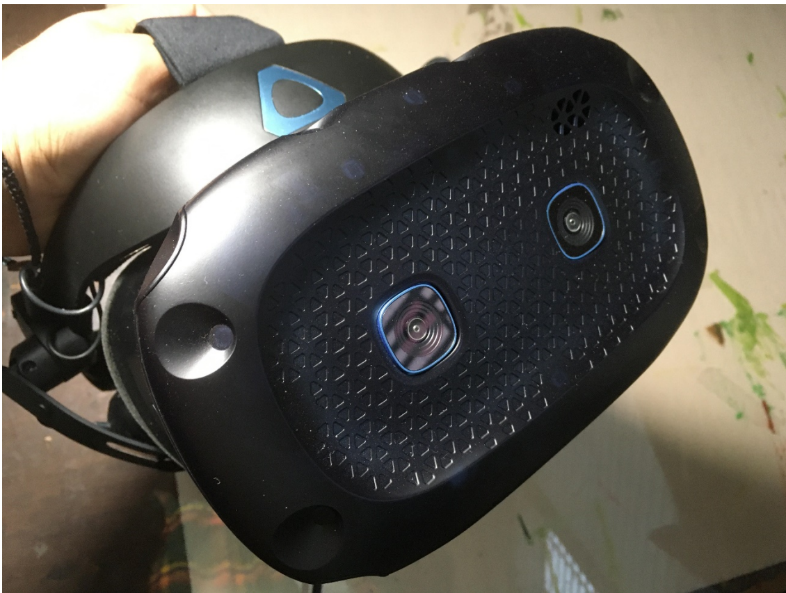
Figure 56: Author's photo of the HTC VIVE COSMOS ELITE used in this thesis VR film.
